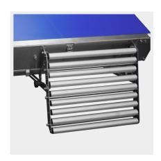
**EXIT RAMP FOR EJECTED**
