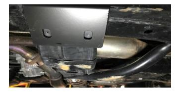
6)Once you have completely aligned and partially threaded in all hardware ((10) 8mm bolts with washers, (2) 3/8 threading screws, and (1)  $3/8" \times 4 \frac{1}{2}"$  bolt with washers and nut) align your e-brake bracket into its original position over the top of the Rock slider mounting plate. Using another 8mm bolt with flat washer reinstall the e-brake bracket only partially threading your bolt into place.
