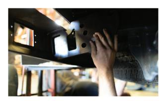
**13.** The electrical connectors can now be reconnected. You can wire the flush mount LED into the reverse lights or they can be wired separately on their own switch.
