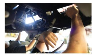
**5.** Disassemble factory bumper to remove wire harness, backup sensors (if applicable) and reverse light.
