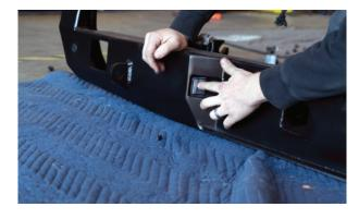
**9.** Install tow plug, use a screwdriver to pull tab out until it snaps. Pull tab up from center
