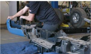
**4.** It may be necessary to use a pry bar to slide the bumper back.
