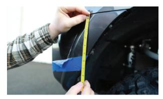
The very top of the cut at the wheel well should end about 5 1/4" down from the top of the plastic bumper just under the second screw holding the bumper to the fender liner.
