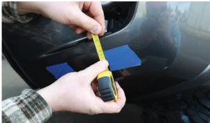
The lower cut line should be 1" below the angled cutout where the fog light is recessed into the bumper and extend inwards towards the AP Low Profile Bumper.
