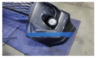
Extend a straight line between the lowerline and the upper end point at the wheel well.
