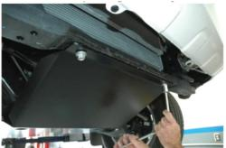
3. (Vehicles with Differential Drop Kits): For some models using a differential drop kit it may be necessary to install the 2 supplied spacers. The spacers go onto the front mounting pedestals. Longer hardware is include for all mounting locations when using differential drop spacers. If rubbing occurs with bracket shown in photos it may be necessary to sand the corner down slightly. We have not had to do this in our builds
