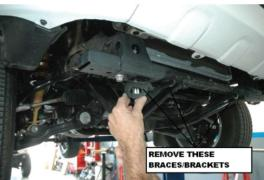
3. (Skip to next step for vehicles with Differential Drop Kits): Install All-Pro skid plate in place of the factory skid plate. Factory hardware will be used in front 4 holes and supplied M8 bolts will be used in rear holes.
