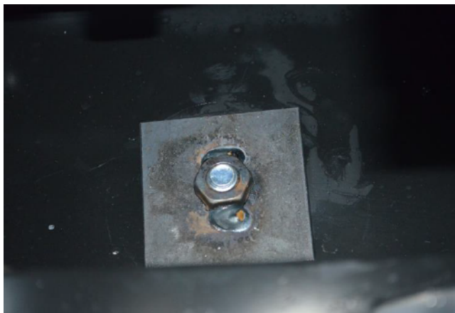
Nut plate on backside of frame covering rectangular hole.
