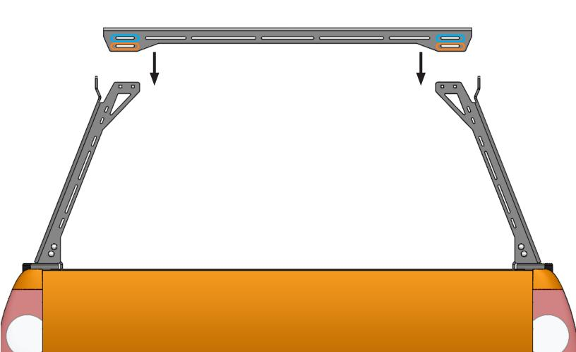
Required Components: **8x** 1/4"-20 Socket button **8x** 1/4"-20 Nylock nut **8x** 1/4" Flat washer
