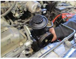
**STEP 9** Install new pump bracket.
