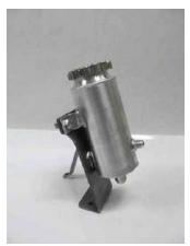
**STEP 9** Fasten to inner fender with 3 8mm bolts and nuts.
