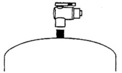
Note: Do not tamper with the air valve on the storage tank. It has been preset and screwed on with blue cap by the manufacturers.
