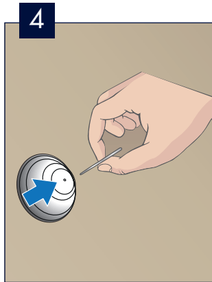
Clean the hole on the bottom with a toothpick
