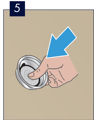
Insert the perforating filter pushing it as far as it goes
