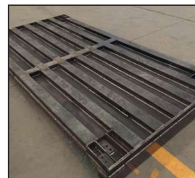
Continuous welding Multiple steel channels
