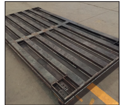
Continuous welding Multiple steel channels
