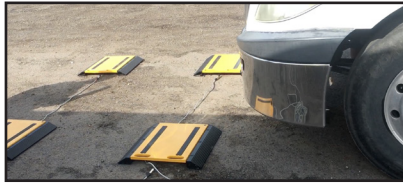
Place pads in proportion to wheel spacing
