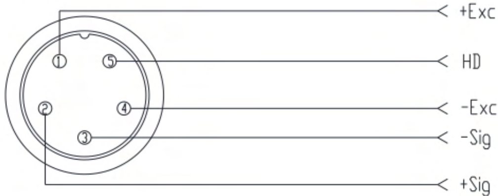
Load cell interface definition
