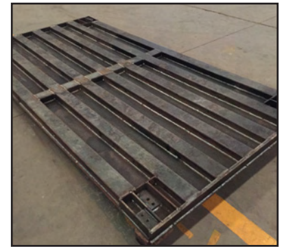
Continuous welding Multiple steel channels
