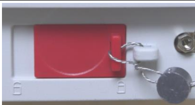
Locked with Wire Seal
