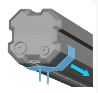
T-bolts should slide into T-channel.
