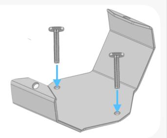
Slide mounting brackets with T-bolts onto the end of the rack shower.
