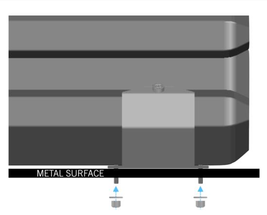
When mounting your Rack Shower to a metal surface, just attach the washers and locknuts.
