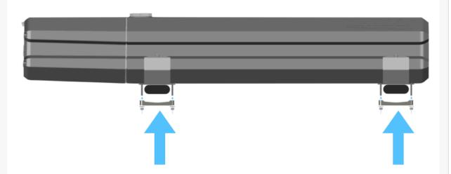
Attach mounting bracket clamp. Then attach and tighten down washer and locknut.
