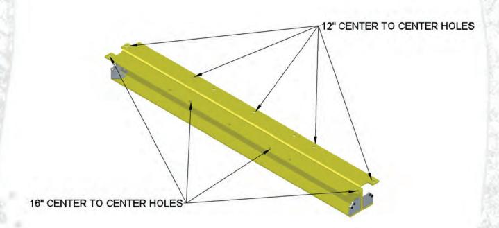
STEP 1: DETERMINE YOUR CEILING JOIST SPACING AND LOCATE THE CENTER OF A JOIST.
