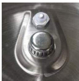
The valve cover is under the inner lid.
