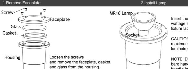
Insert the lamp with the correct wattage and type marked on the fixture label.
