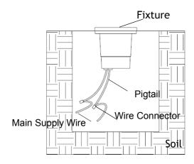
Strip both leads from the luminaire pigtail. Using two wire connectors (sold separately), connect the leads from the luminaire to main supply cable leads.
