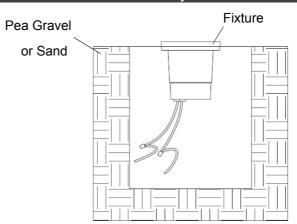
Install the fixture in the hole and fill the extra space with pea gravel or sand for proper water drainage.
