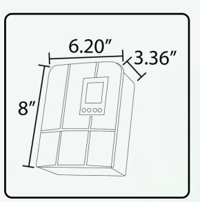
**POWER: CERTIFICATE:** 300W AC 12V **ETL LISTED FINISH: BODY: HEAVY DUTY** BLACK **FEATURE:** PLASTIC BODY **BUILT - IN PHOTOCELL** WATERPROOF RATING: AND ASTRONOMIC TIMER **IP65 TSP300 SPEC SHEET**
