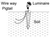
Clear away an area in the ground at the wire way on top of the stake. Lay the luminaire pigtail into the wire way and attach the luminaire onto the stake. Tighten until snug.
