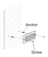
Note: Anchors are required for concrete or brick walls. Hold the luminaire on the wall and mark two points for the anchors using the mounting holes as guides. Then drill the proper holes using the marks. Insert the anchors into the drilled holes.
