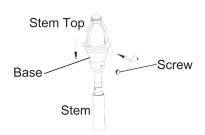
Place the Base over the bulb and thread the stem top onto the stem. Hand tighten Screw until snug.
