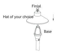
Place the hat of your choice onto the stem top and secure it with the finial. Hand tighten until snug.
