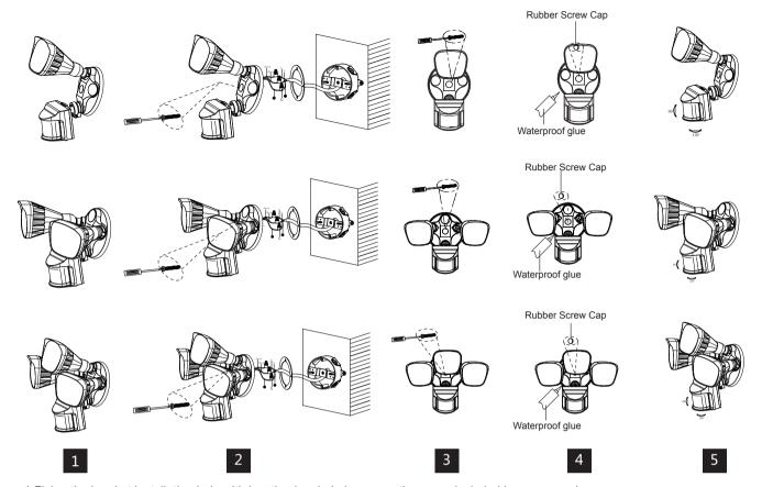
1. Fixing the bracket installation hole with junction box hole by screw, the screw included in accessory bag.
