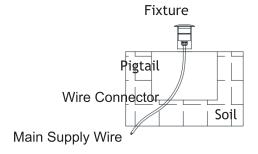
Strip lead from the luminaire pigtail. Using wire connectors (sold separately), connect the leads from the luminaire to main supply cable leads.
