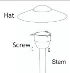
Loosen the hat and remove it from the top end of the stem by pulling it up and over the bulb.
