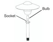
Insert the bulb with the correct wattage and type marked on the luminaire label.
