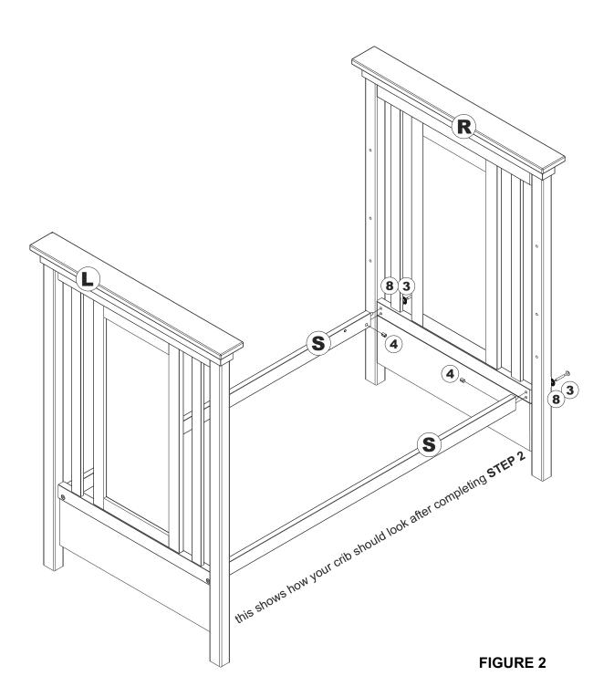
Attach the right panel **(R)** to the part of the crib resulted after **STEP 1**, using the same technique. Do not tighten completely the bolts at this step, you will be asked to do this later.
