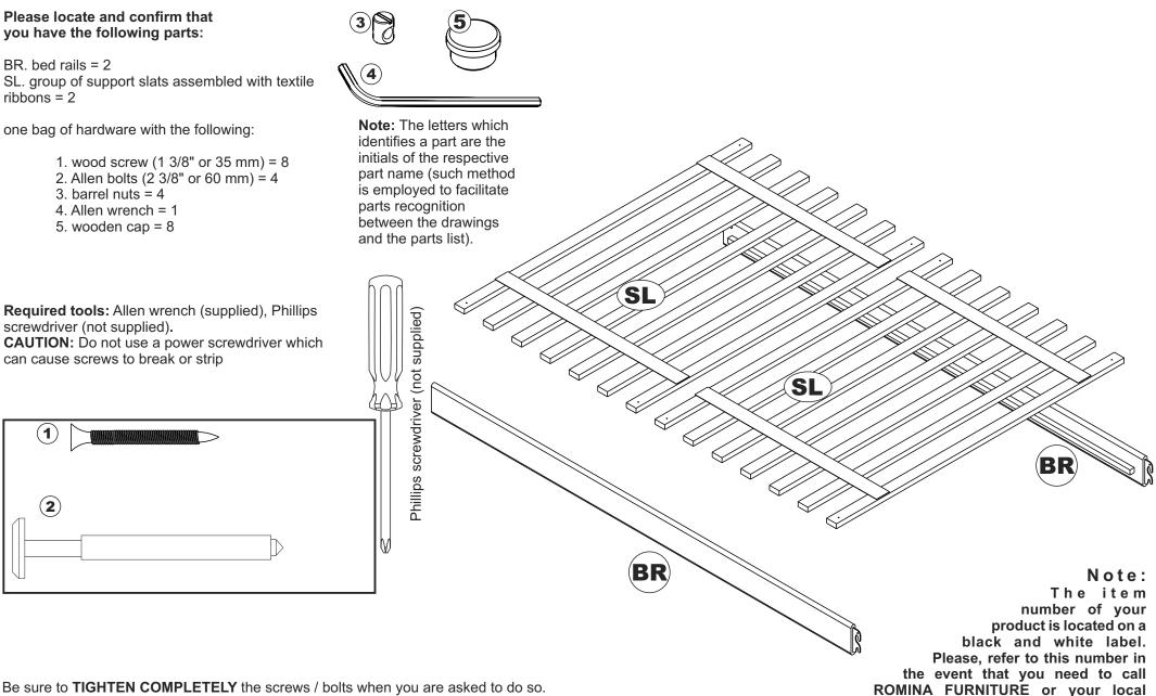
Be sure to TIGHTEN COMPLETELY the screws / bolts when you are asked to do so.
