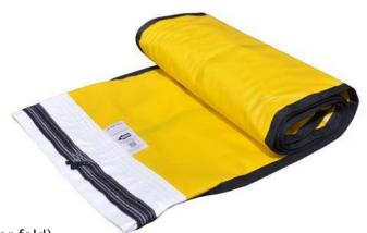
**Materials: Outer Layer:** 18oz. PVC Coated Polyester or 1000 Denier Nylon Fabric (1000 Denier x 1000 Denier) with a 1 oz. Urethane coating on the inside and a DWR finish on the outside (water repelant).
