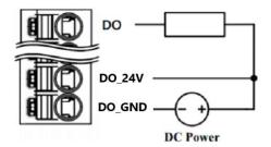
EG500 provide 6x DO to control the external slave devices. With an overvoltage protection circuit that DO 24V wiring, it could filter the overvoltage to avoid destroying device itself.
