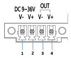
EG500 right side panel provide a 4-pin terminal block connector for Power input and a bridge connection for power output. The defination of PIN 1 "V-" as GND, PIN 2 "V+" for  $9V^{3}6V$  DC input. While PIN 3 & PIN 4 is a parallel power from PIN 1 & PIN 2, which considering designed for slave devices power supply.
