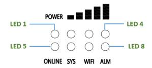
EG500 extend 8 LED indicators for apparent status indication as printed label shown,
