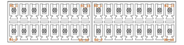
EG500 provides two terminal blocks for expanded I/O ports, the ports PIN defination as shown as the printed label above terminal block accordingly.
