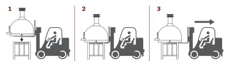
When setting the oven on a stand, **place the stand first**, then place the oven on top. Keep forks centered between the stand-legs to ensure the oven is properly aligned and square with the stand.
