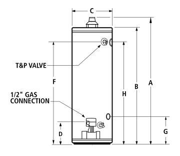
Maximum Hydrostatic Working Pressure: 150 PSI
