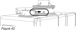
2. Remove and discard the combustion air vent
