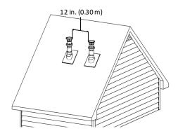
Figure 25: Between terminals at same level
