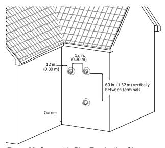
Figure 22: Concentric Pipe Termination Clearances
