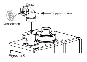
5. Install the exhaust vent pipe. Ensure it is properly seated. Secure the exhaust vent pipe to the exhaust
