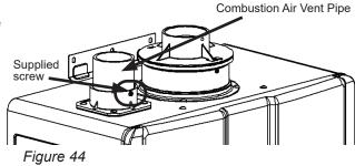
4. Place the vent screen or room air screen inside elbow and secure with the supplied screw. Use the room air screen for environments where room air is dusty (Figure 45).
