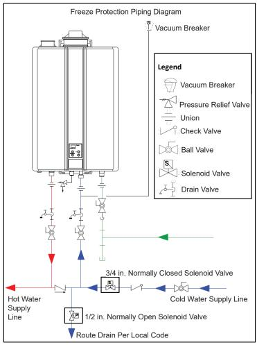
Figure 7: Freeze Protection Piping Diagram
