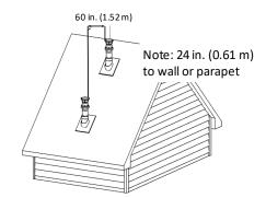
Figure 24: Between terminals at different levels
