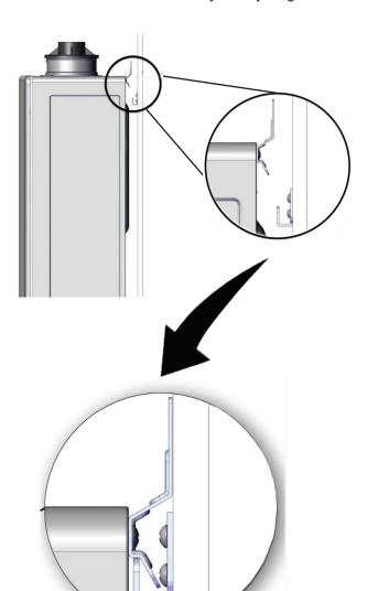
Figure 11: Mount the top bracket
