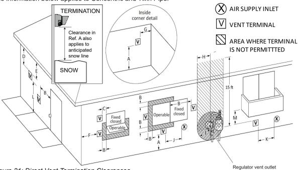
Figure 21: Direct Vent Termination Clearances
