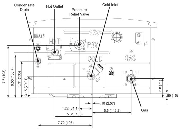
Figure 6: Supply Connections
