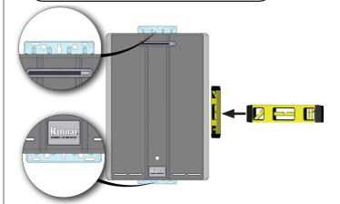
Figure 13: Mount the water heater
