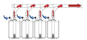
Figure 20: Common Vent, Room Air
