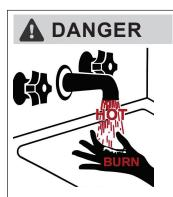
Water temperatures over 125°F (52°C) can cause severe burns or scalding resulting in death.
