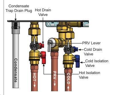
Figure 96: Piping Diagram
