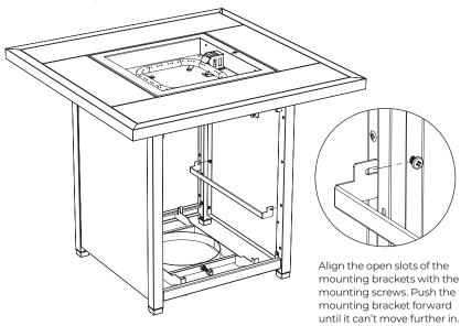
Tighten both mounting screws.
