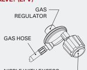
NIPPLE WITH EXCESS FLOW LIMITING DEVICE (EFV)
