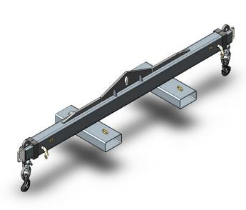
The type CFL-2439 Spreader Beam is a unique multitasking Beam which can be used by Crane or Forklift to lift long loads. Using a Crane, loads can be lifted via the centre single hook point (as a 'Lifting Beam'), or end lifted using a 2 leg Chain Sling (as a 'Spreader Beam'). If lifting by forklift, the 600mm long slipper pockets allow for fast and safe connection to the truck.
