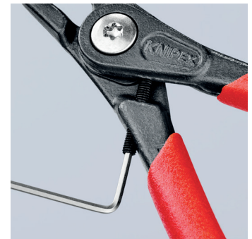
Overstretching limiter with screw stop prevents overexpansion of circlips
