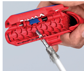
Stripping the internal portion of the coax cable
