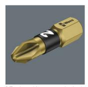
bits BiTorsion are absolutely premium products. They have a softer BiTorsion zone which reduces the hardness of the shaft by about 20 % in comparison to the drive tip. This means that the peak loads that cause bit breakage and premature wear are absorbed in this zone - something which enhances the service life of the bits.
