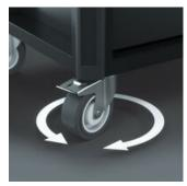
two swivel castors The are equipped with a double stop: The locked castor reliably prevents it from rolling away, the locked spindle carrier prevents the turning castors from unintentionally, e.g. on sloped surfaces. The oil- and acidresistant elastic wheels ensure smooth running. A protective ring prevents the ingress of dirt and threads.
