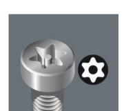
TORX® tools with a borehole prevent the unauthorised unfastening of safety screws. The screws contain a pin that protrudes into the drive profile so that "normal" TORX® tools cannot be used. This pin fits into the borehole of TORX® BO tools allowing safety screws to be unfastened.
