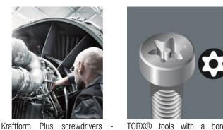
TORX® tools with a borehole prevent the unauthorised unfastening of safety screws. The screws contain a pin that protrudes into the drive profile so that "normal" TORX® tools cannot be used. This pin fits into the borehole of TORX® BO tools allowing safety screws to be unfastened.
