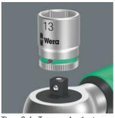
The Safe-Torque A 1 torque wrench has 1/4" square head mounting and is suitable for 1/4" sockets.
