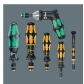
Wera torque screwdrivers. With a factory pre-set torque value set to the smallest scale value. For all applications, where the same constant torque and repeat accuracy are required. The torque can be changed with an extra tool within the measuring range (recalibration kit can be ordered with the code number 05137004001). Afterwards you can check the set value using an off-the-shelf torque tester.
