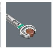
The Joker's clever double-hex geometry delivers a very positive connection with nuts or bolts - it's a perfect fit. And the exchangeable, hardened metal gripping plate in the Joker's open end literally bites itself into the bolt, with its extremely hard tips. Both features combine to prevent slipping, even at higher torque. 6000 Joker Ratcheting combination wrenches
