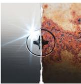
Stainless steel has the property of not rusting. However, if tools made out of conventional steel are used for stainless steel components or screws, the particles left behind from these tools can adhere to the surface and then rust. This effect - known as extraneous rust - can impair the visual appearance and even cause structural damage that may result in expensive repair work. The wear particles that cause this rust effect can be prevented by using stainless steel tools.
