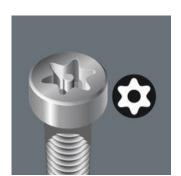
TORX® tools with a borehole prevent the unauthorised unfastening of safety screws. The screws contain a pin that protrudes into the drive profile so that "normal" TORX® tools cannot be used. This pin fits into the borehole of TORX® BO tools allowing safety screws to be unfastened.
