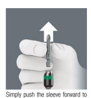
change the bit. The spring mechanism lifts the bit off the magnet and unlocks the tool. The bit can be easily removed. The rapid-out function makes it easy to remove even the smallest bits without extra tools.
